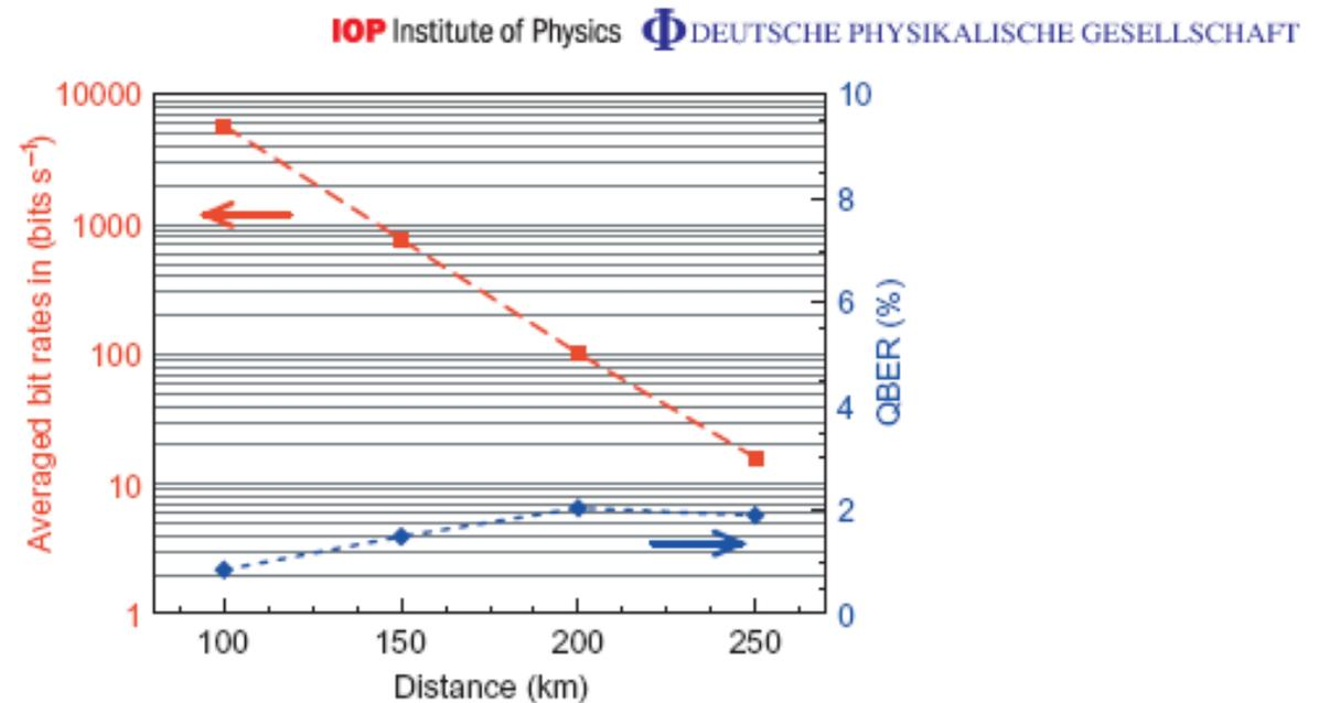
Figure 6. Averaged secret bit rates (red squares) and QBER (blue diamonds) for a range of SMF-28<sup>®</sup> ULL fibre lengths.
