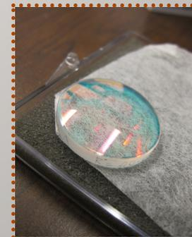
We use a stable monolithic cavity for frequency filtering
