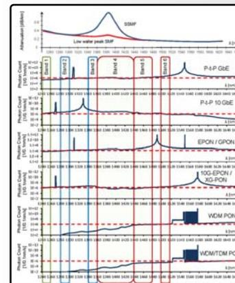
Raman, FWM, Rayleigh scattering have been simulated when classical signals are applied to a 40 channel network. The tolerable background for a possible QKD signal is assumed to be 600000 Photons
