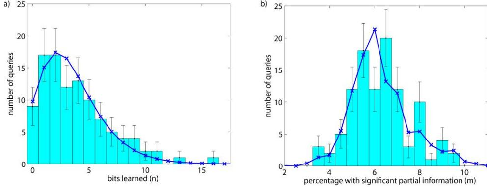
**Figure 2** – Histogram of experimental (bars) and simulated (crosses) private query results for  $\mu=9.5$ . **a)** Number of bits learned by Ursula (i.e. with an error rate less than  $10^{-3}$ ). **b)** Percentage of the database where Ursula has significant partial information (i.e. with an error rate less than  $1/3$ ).
