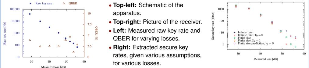
We achieve QKD with up to 56 dB of loss while *including finite-size effects* over 20 min collection.
