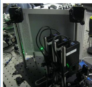
We are investigating a possible spin-off for high-loss-tolerant QKD: via a **diffusive screen**. This could allow the development of *simple, wireless, multi-access QKD hot-spots* for mobile devices.
