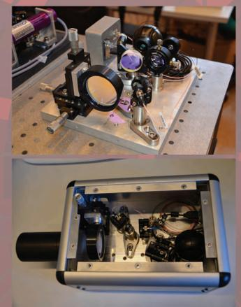
Usage of commercial fiber connections for dark channel encounters, however, a problem with polarization mish-mash produced by accidental birefringence of fiber due to strain in welding and fiber flexion regions.
