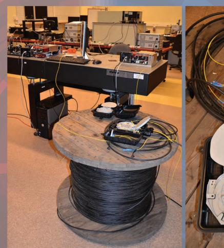
Tests of the system using different probe optical fibers for a dark quantum channel and compare QBER to short (2-m) polarization fiber connection. Testing include also a commercial 5 km long patchcord of fibers to assess possibility of practical implementation of entangled QKD system in metropolitan real network.
