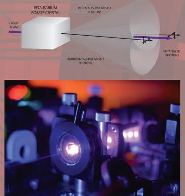
The AIT EPR Quelle systems are equipped with telescope setups design for allowing long distance QKD (up to 5 km) in open air dark channel, where the satisfactory level of conservation of polarization of flying qubits is provided
