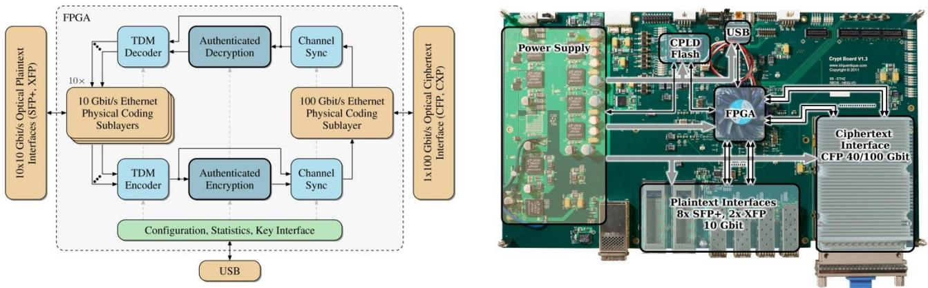
Fig. 2: High-level block diagram of the 100 Gbit/s encryption system. Right: 1<sup>st</sup> prototype PCB of the system.
