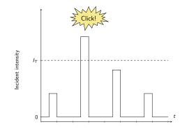
This trick prevents a single-photon detector from seeing incoming pulses below an intensity threshold  $I_T$ . Only the second pulse will give a click.
