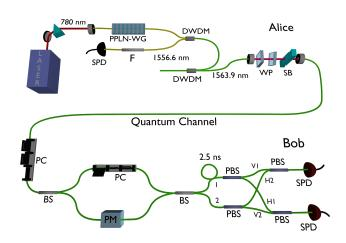
FIG. 2. Experimental realization of the proof-of-priciple ddiQKD protocol. Labelled components include, dense wavelength division multiplexers (DWDM), bandpass filter (F), waveplates (WP), Soleil-Babinet compensator (SB), polarization controllers (PC), phase modulator (PM), 50/50 beam splitters (BS), polarizing beam splitters (PBS) and single-photon detectors (SPD).
