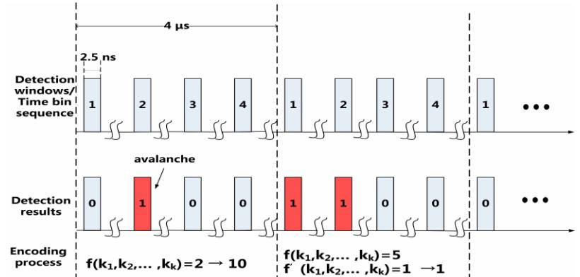
Fig. 1: (Color online) The schematic graph of encoding process in time sequence, where  $N = 4$ .
