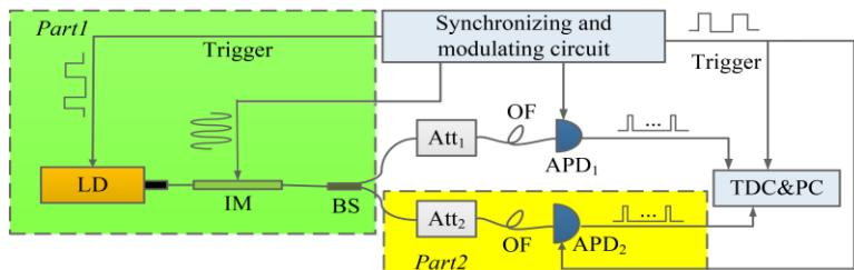
Fig. 2: (Color online) Schematic setup of the experiment. A pulse LD with the wavelength of 1550 nm was used as an optional light source and was triggered by 1 MHz electronic pulses. LD: Laser diode; IM: optical intensity modulator; BS: beam splitter; Att: electronically variable optical attenuators (EVOA); OF: optical fiber; APD: avalanche photodiode; TDC: time-to-digital converter; PC: personal computer.
