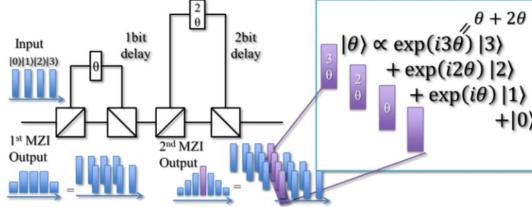
Figure 1 : Concept of projection measurement with cascaded delay MZIs.
