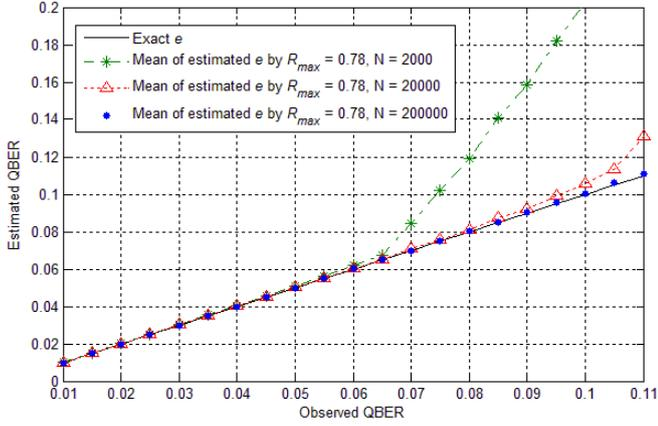
Fig. 3. Estimated bit error rate  $e$  by the ML estimator as a function of observed QBER.
