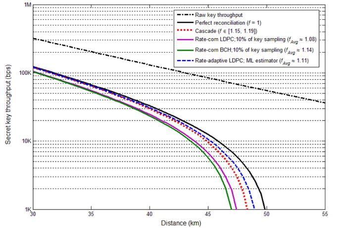
Fig. 5. Secret key throughput as a function of distance. This simulation is calculated by 1 GHz clock rate of the source over  $\alpha = 0.2$  dB/km,  $\eta = 0.1$ ,  $p_d = 10^{-5}$ , and  $q = 0.5$ .
