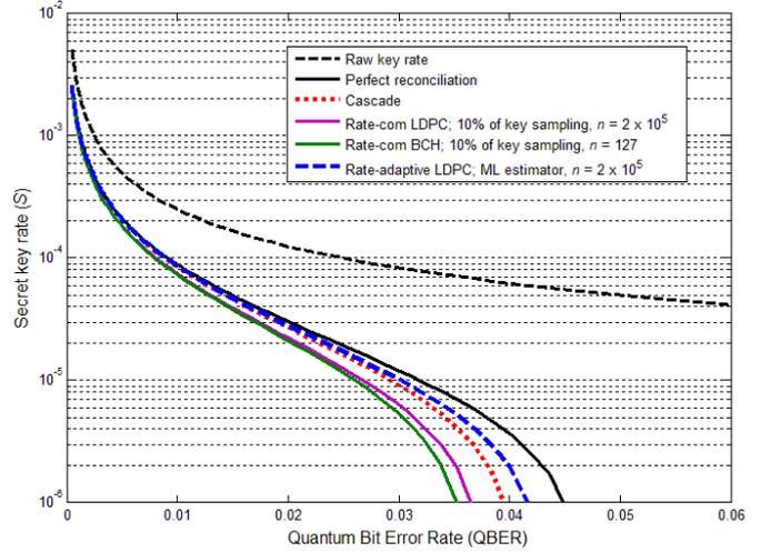
Fig. 4. Secret key rate  $S$  as a function of QBER. This simulation is calculated by  $\alpha = 0.2$  dB/km losses in optical fiber, a detection efficiency of  $\eta = 0.1$ , a dark counts probability of  $p_d = 10^{-5}$ , and  $q = 0.5$ .
