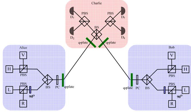
Figure.1. A schematic of our modified MDI-QKD protocol.
