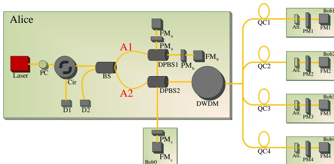
Fig.1. Schematic of multi-user system for quantum cryptography with wavelength division multiplexing. Laser: pulsed laser diode; PC: polarization controller; Cir: circulator; DPBS:
