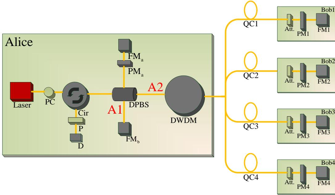
Fig. 2. Schematic of multi-user system with by phase coding and polarization measurement. Laser: pulsed laser diode; PC: polarization controller; Cir: circulator; DPBS: Four-port polarization beam splitter; PM: phase modulators; FM: Faraday mirrors; QC: quantum channel; P: linear polarizer at  $+45^\circ$ ; D: single photon detectors; Att.: attenuator; DWDM: dense wavelength division multiplexing.
