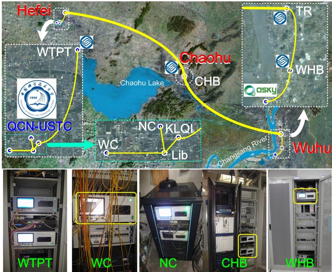
**Fig.1** Geographic distribution and photographs of the wide area QKD network. Hefei, Chaohu, and Wuhu are three cities, and nodes WTPT, CHB, TR and WHB are telecommunication nodes belonged to China Mobile Ltd. Nodes WC, NC, Lib and KLQI compose the quantum campus network of University of Science and Technology of China (QCN-USTC).
