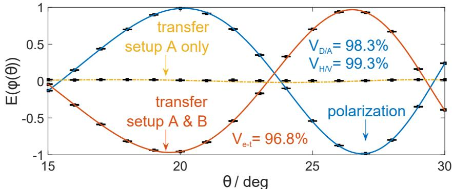
**Figure 2:** Experimental results. Two-photon correlation functions  $E(\phi(\Theta))$  in the polarization (blue) and energy-time (red) DOF as a function of the variable phase shift  $\phi(\Theta)$  introduced in Alice’s measurement module. Almost no interference was observed when the energy-time to polarization transfer setup was introduced in Alice’s detection module only, thus excluding single-photon energy-time coherence.
