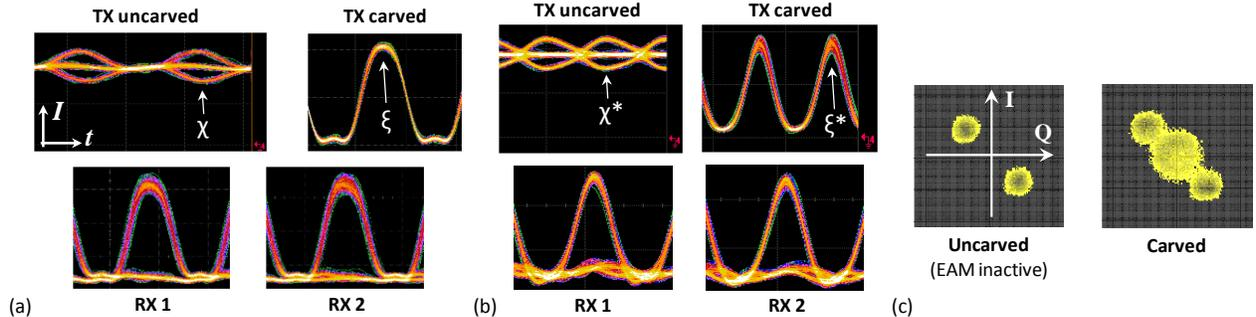
**Fig. 2.** Eye diagrams after transmitter (TX) and receiver (RX) for (a) DML+MZM and (b) EML. Eye diagrams after the transmitter are shown in absence and presence of carving, while receiver eyes are shown for present carving. (c) Constellations in I/Q phase space retrieved by modulation analyser for EML-based transmitter. The carved constellation has been sampled at twice the modulation symbol rate.
