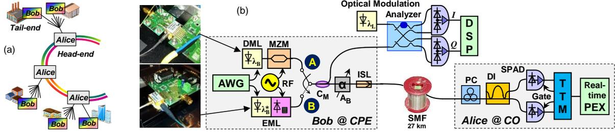
**Fig. 1.** (a) Network context. (b) Experimental setup for DPS-based QKD with low-complexity transmitter at Bob.
