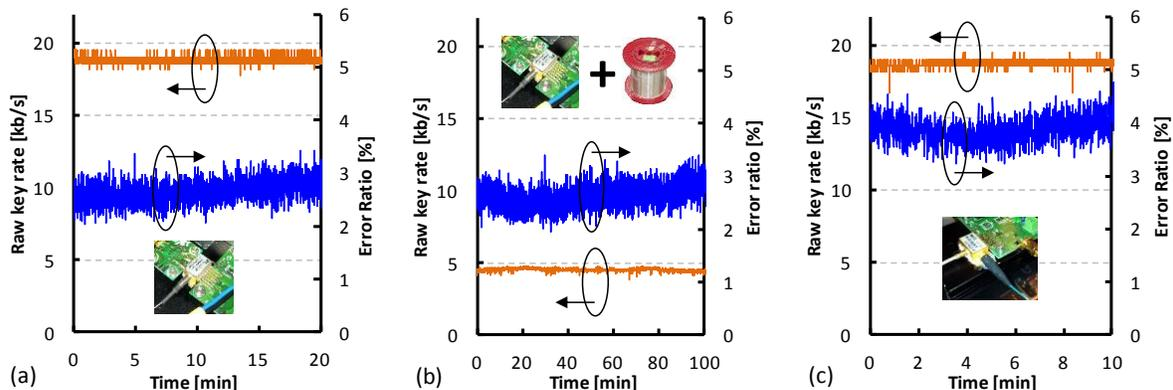
**Fig. 3.** QBER (blue) and raw key rate (orange) for (a) DML+MZM and back-to-back transmission and (b) over 27 km SMF fibre span, (c) integrated EML and back-to-back transmission.
