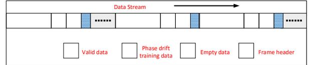
FIG. 1. Sample data flow of the CVQKD system
