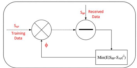
FIG. 2. Schematic of the high precision phase compensation
