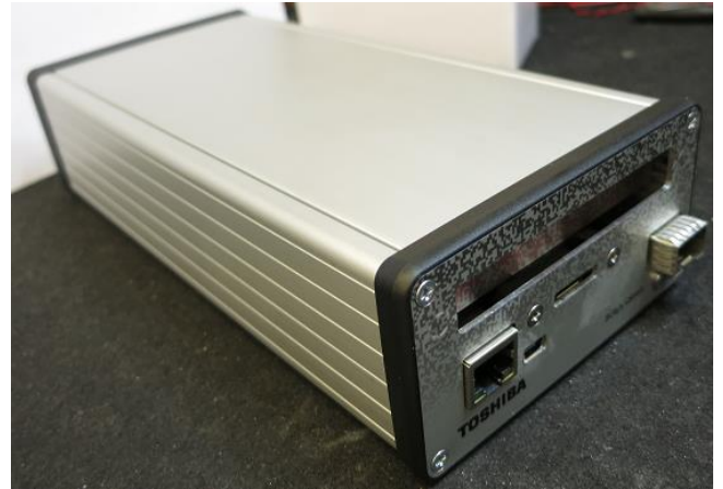
Figure 1: The Toshiba QRNG. The device has dimensions of 10 x 23 x 5 cm.
