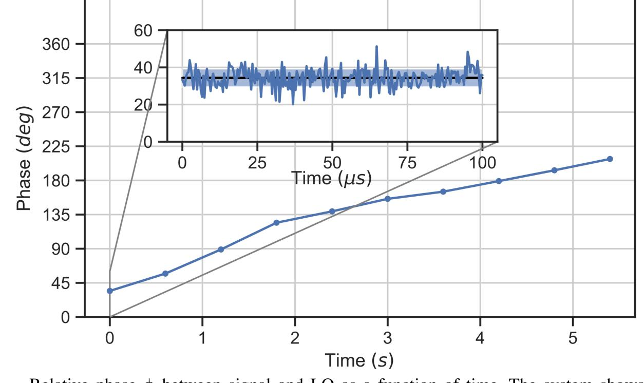
Relative phase  $\phi$  between signal and LO as a function of time. The system shows a drift of about 32 deg/s, while for time scales comparable with the chunk size no drift is observed (see inset).
