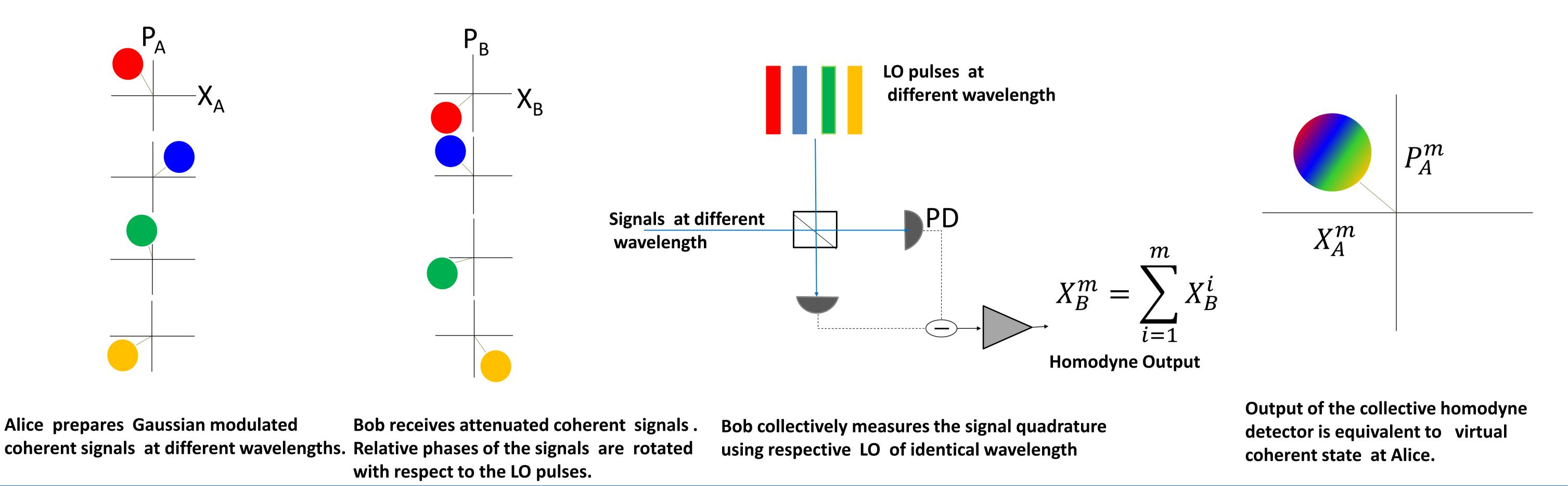
**Results** – Collective detection of multi-mode signals effectively reduces the contribution of electronic noise.
