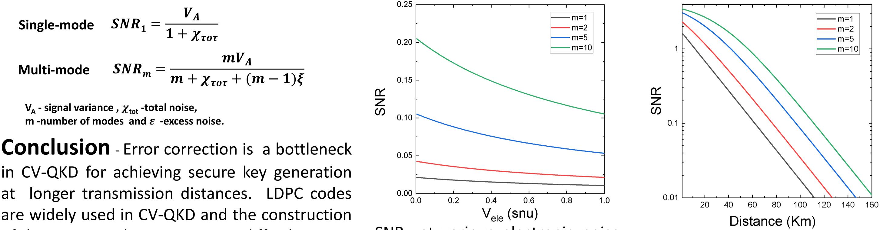
in CV-QKD for achieving secure key generation at are widely used in CV-QKD and the construction of these , at very low SNR, is very difficult. Using multi-mode signals with collective quadrature detection can increases the SNR in CVQKD and the overall transmission distance . improves With m=5, the SNR is increased by 5 times and the transmission distance by 30 percent.
