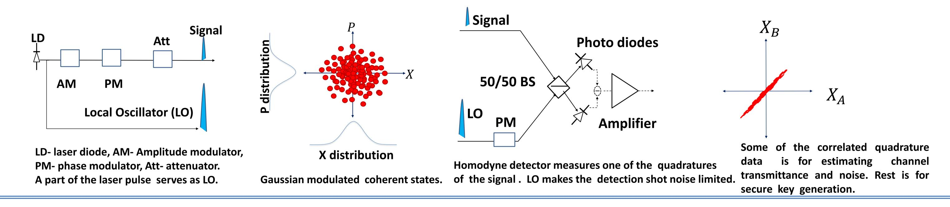
**Multi-mode CV-QKD** – Alice prepares multiple wavelength signals each with random quadrature modulation.
