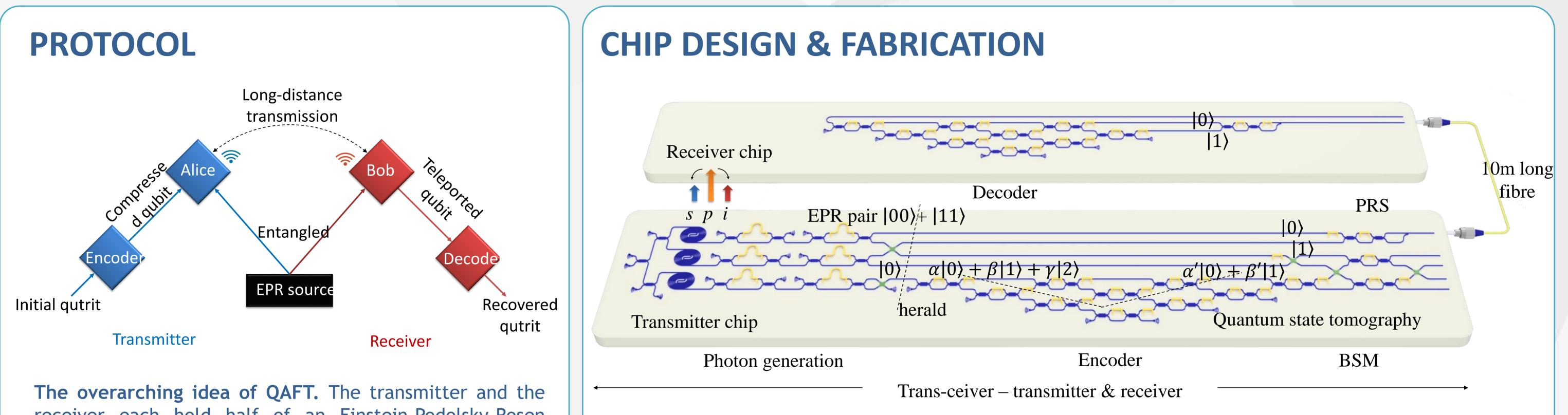
receiver each hold half of an Einstein-Podolsky-Rosen (EPR) pair. At the transmitter, the initial qutrit is compressed into qubit by the trained encoder, and BSM is performed. Depending on BSM results and the encoder, the receiver will set up the decoder and reconstruct the initial qutrit from the teleported qubit.
