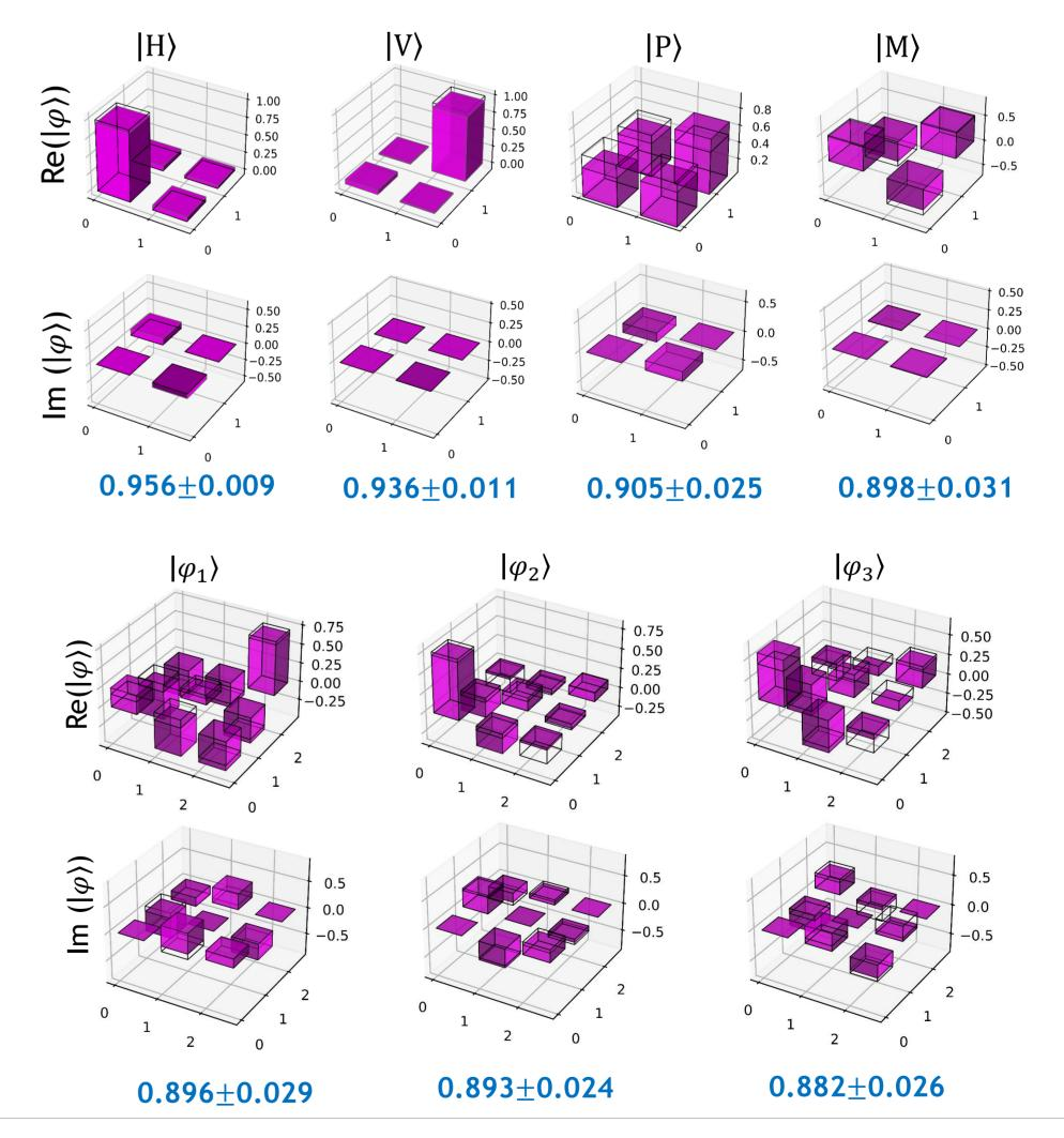
Chip-to-chip teleportation results. The teleported qubit was decoded to recover the original generated qutrit on the receiver chip, with a fidelity of  $0.894 \pm 0.026$ .
