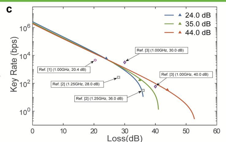
**c.** Finite-key secret rate versus different channel loss with 125 MHz system frequency and the comparison with the state of the art MDI-QKD experiments.
