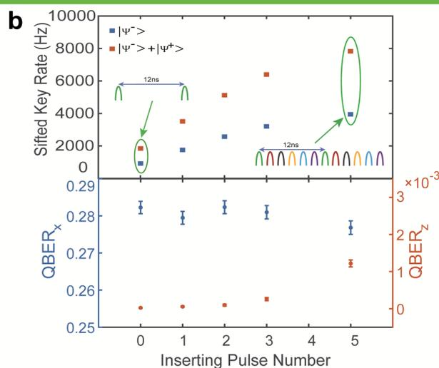
**b.** Sifted key rate with only  $|\Psi^- \rangle$  measurement or two Bell state measurement versus inserting pulse number and the measured QBER in X-basis or Z-basis versus inserting pulse number.
