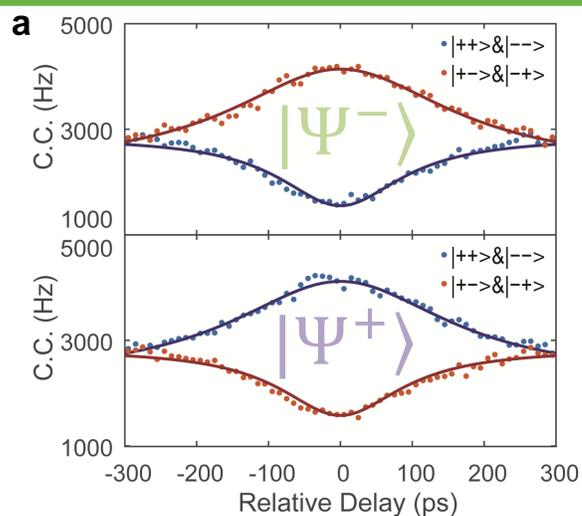
**a.** The two-photon coincidence counts with BSM as a function of relative electronic delays between Alice's and Bob's pulse sequence.
