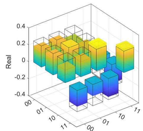
Real part of reconstructed density matrix for state  $|0\rangle + |1\rangle$  with error at 2<sup>nd</sup> qubit. The fidelity is measured to be  $F = 0.8522$ .
