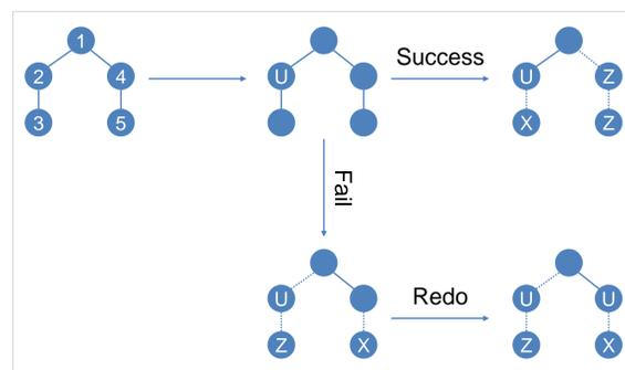
Scheme of error corrected teleportation. The initial state  $|L_5\rangle$  allows us to reconstruct the basic entangled state  $|0\rangle + |1\rangle$  if the teleportation fails.
