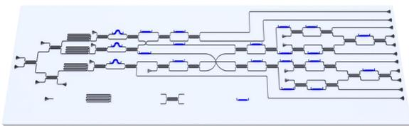
Schematic of photonic integrated chip for error-correction. The single photon is generated on chip via the SFWM and the quantum state is encoded and measured in the linear optical circuit part.
