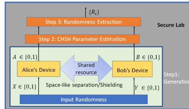
Figure 1. Sketch of a typical DI protocol for randomness expansion.
