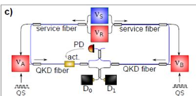
c) **Our approach:** an additional sensing laser, with frequency  $\nu_S$  travels the service fiber with the reference laser, and the QKD fibers together with the QKD lasers
