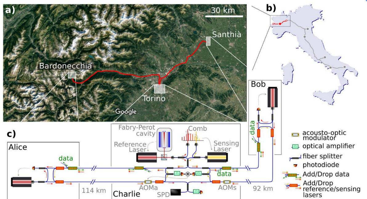
a) The testbed layout, with the Charlie node located at INRIM (Torino) and the Alice and Bob nodes in Bardonecchia and Santhià b) A sketch of the Italian Quantum Backbone c) The experimental setup.
