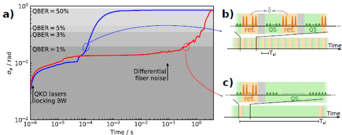
a) Deviation of the phase  $\sigma_\phi$  between the two QKD lasers interfering in Charlie at different timescales, in an unstabilized (blue) and stabilized (red) condition. The shadowed areas indicate upper thresholds for relevant values of the QBER. The interferometer must be realigned after 100  $\mu$ s and 0.4 s for a QBER=1% using an unstabilised or stabilised interferometer respectively
