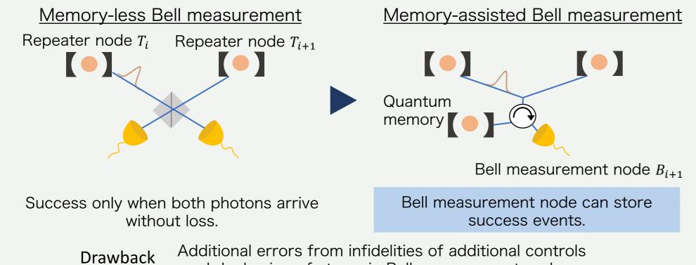
By increasing the number of memories, the memory-assisted Bell measurement can overcome the memory-less Bell measurement with the current parameters.
