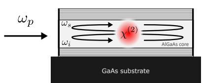
A pump beam illuminates an AlGaAs waveguide where photon pairs are generated by SPDC.
