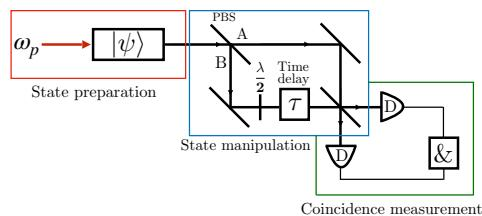
HOM interferometer. A time delay performs a one qubit gate
