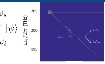
Simulated JSI of the state emitted by the nonlinear cavity (left). Experimental JSI, with stimulated parametric down conversion (right)
