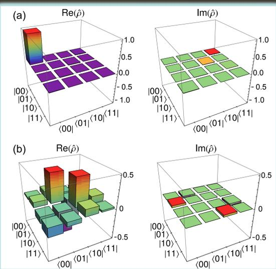
**Figure 4:** The real (Re) and imaginary (Im) parts of the reconstructed density matrices of the generated states measured by quantum state tomography using the setup in Fig. 2 for (a) type-0 SPDC source (b) type-2 SPDC source, respectively. Here “0”  $\equiv |V\rangle$  and “1”  $\equiv |H\rangle$ .
