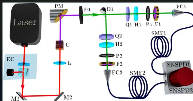
**Figure 2:** Generation and full tomography of polarization entangled photons at 2.1  $\mu\text{m}$ .
