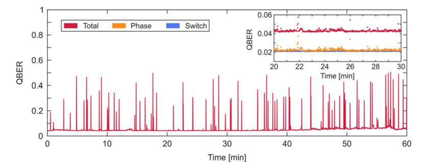
Phase lock-loop performance over 10 Km of multicore fiber.
