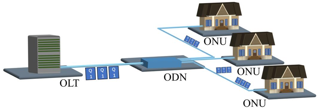
Fig. 1 Example of a downstream access network. Signals from the optical line terminal (OLT) are sent to the optical distribution network (ODN), and then passively distributed to multiple optical network units (ONUs) through the beamsplitter (BS).
