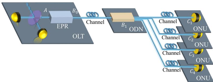
Fig. 2 Entanglement-based (EB) model of a CV-QKD downstream access network.
