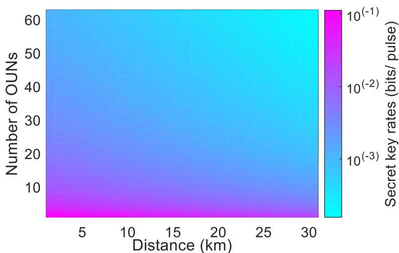
Fig. 4 Achievable secret key rates against the number of ONUs access in the network and transmission distance. The secret key rates are represented by the pseudo-colors. Simulation parameters: variance of the EPR state  $V=5$ , channel excess noise  $\epsilon=0.05$  (SNU), detection efficiency  $\eta_d=0.6$ , electronic noise  $\eta_e=0.99$ , and reconciliation efficiency  $=0.956$ .
