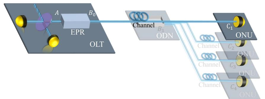
Fig. 3 Modified EB model which is applicable for the security analysis for the downstream access network. Only the OLT and the specified ONU are highlighted.
