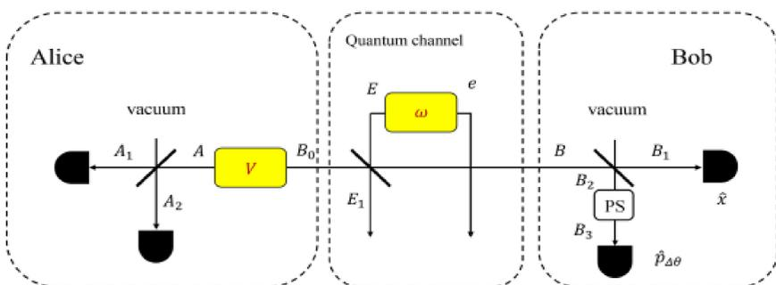
Fig. 2. The EB description of measurement angular error in CV-QKD scheme using heterodyne detection.
