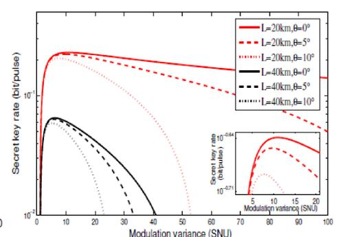
Fig. 4. The optimal modulation variance for the systems with different measurement angular error.
