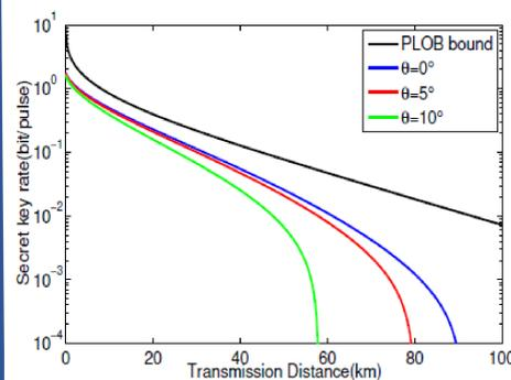
Fig. 3. The secret key rate versus the transmission distance with different measurement angular errors.
