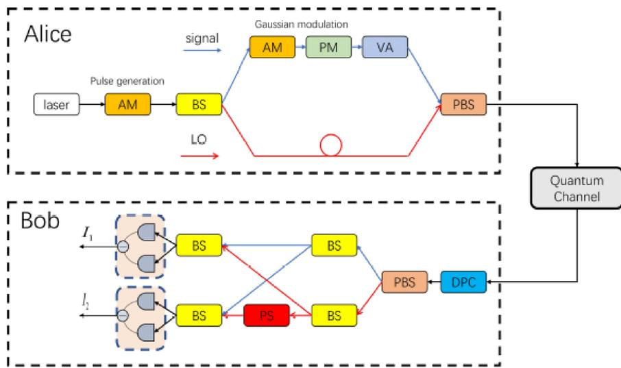
Fig. 1. Schematics layout of the heterodyne detection GMCS protocol. AM: amplitude modulator; PM: phase modulator; BS: beam splitter; PBS: polarization beam splitter; VA: variable attenuator; DPC: dynamic polarization controller; PS: phase shifter.
