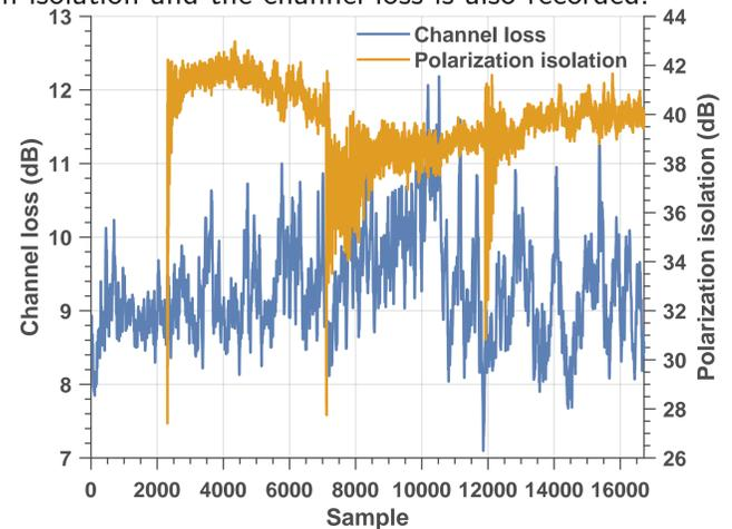
Polarization isolation can be maintained at a high level in spite of channel loss fluctuations.
