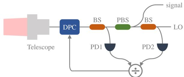
At a receiving terminal, the outputs of the PD1 and the PD2 are divided and used as feedback signals for the DPC. Selecting an optimization algorithm according practical environments and optimizing the feedback.
