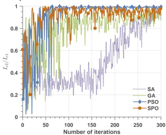
Different algorithms may have different performance in different environments. Most importantly, a suitable algorithm should have fast and nice convergence.
