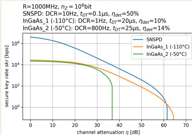
ii. Detector comparison: superconducting nanowire (SNSPD) vs. InGaAs single photon avalanche (SPAD)
