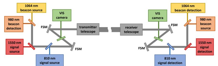
Fig. 6. Optical link architecture.
