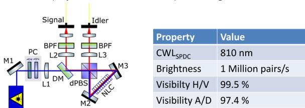
Fig. 3. EPS optical design. Non-linear crystal (NLC) is pumped bidirectionally with 405 nm in a sagnac configuration, generating entangled photon pairs at dual-wavelength polarization beam splitter (dPBS). The SPDC photons are then separated using a dichroic mirror (DM). SPDC photons are then collected in single mode fibers.
