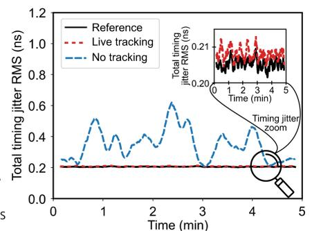
Fig. 7. Comparison of total system jitter with correlated photons and reference for 100 ms data package size and 600 ms feedback loop time. Live tracking of the correlation peak clearly reduces the jitter.
