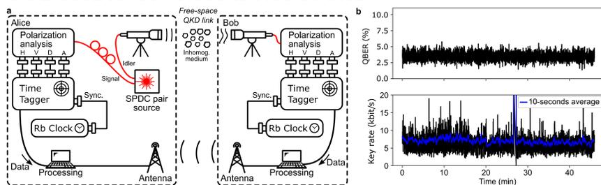
Fig. 1. Quantum key distribution setup **a**, including a spontaneous parametric downconversion source, and telescopes with active tip-tilt beam stabilization. **b** Achieved key rates of 7.1 kbit/s on average and quantum bit error rates (QBER) during 50 min of key exchange on a 300-m free-space link.
