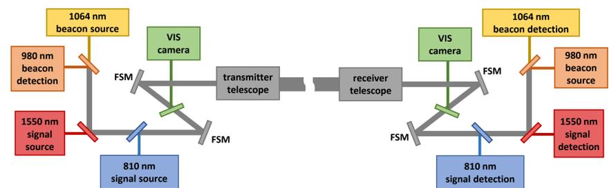
Fig. 6. Optical link architecture.
