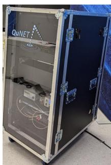
Fig. 4. Rack-integrated EPS with time-tagging and synchronization electronics
