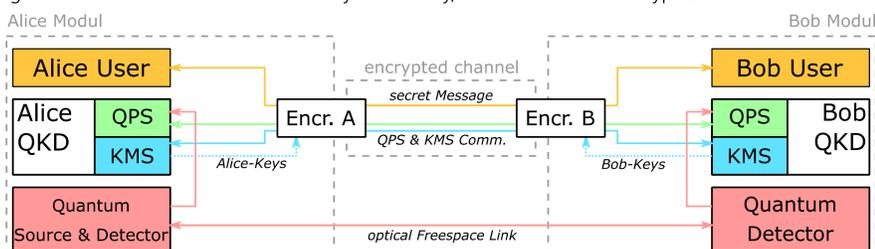
Fig. 2. The two QKD-modules are connected by an optical freespace link for transmission of the quantum signal, as well as through an encrypted classical channel for Quantum-Postprocessing (QPS), Key-Management (KMS) and user communication. The QPS retrieves quantum events and generates the secure key, which is stored in the KMS. The KMS feeds the key to the encryptor (Encr. A/B), which then uses it to encrypt the classical channel.
