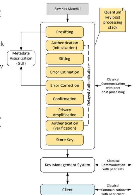
Fig. 8. Illustration of the quantum key distribution software components and their interaction.
