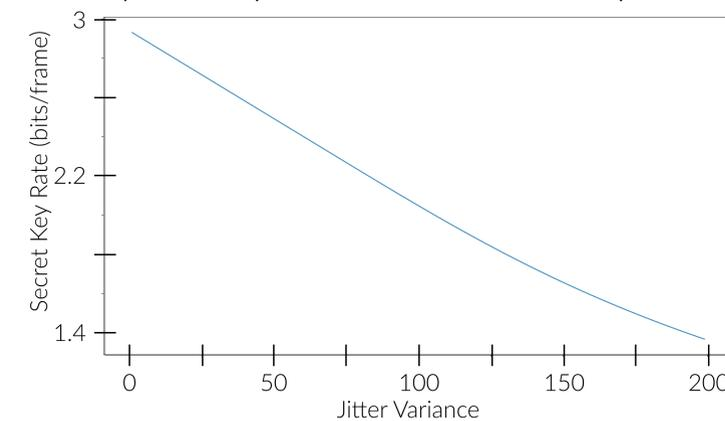
Reed Solomon Codes require  $t$  symbols to resolve  $t$  errors at known locations. Using this, we calculate the number of parity symbols needed to correct the expected errors and subtract these bits from the raw key. Using larger (or fewer) bins can increase the jitter resilience.
