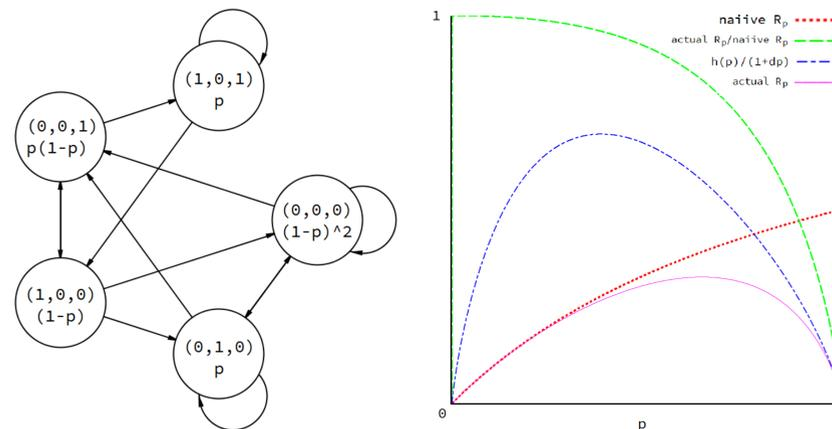
Each state contains an identifier  $(d_i, n_1, d_o)$ , where  $d_i$  and  $d_o$  are recovery-time into and out of the frame, respectively, and  $n_1$  is the number of occupied bins inside the frame, minus one if  $d_o > 0$ . The expression under each identifier is the transition probability of all transitions into that state.
